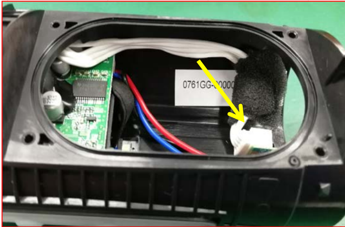
11: Pull out the cable as show
