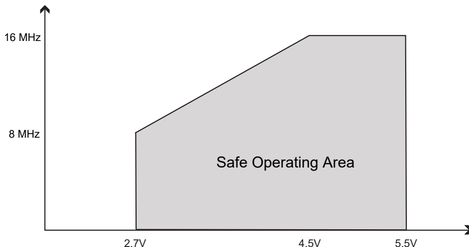
Figure 33-2. Maximum Frequency vs. V_{DD} for [85, 125]^{\circ}\text{C}
