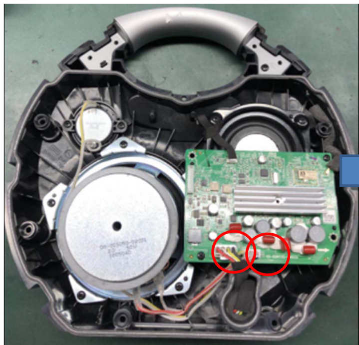
8. Unplug 2pcs cable on the main board
