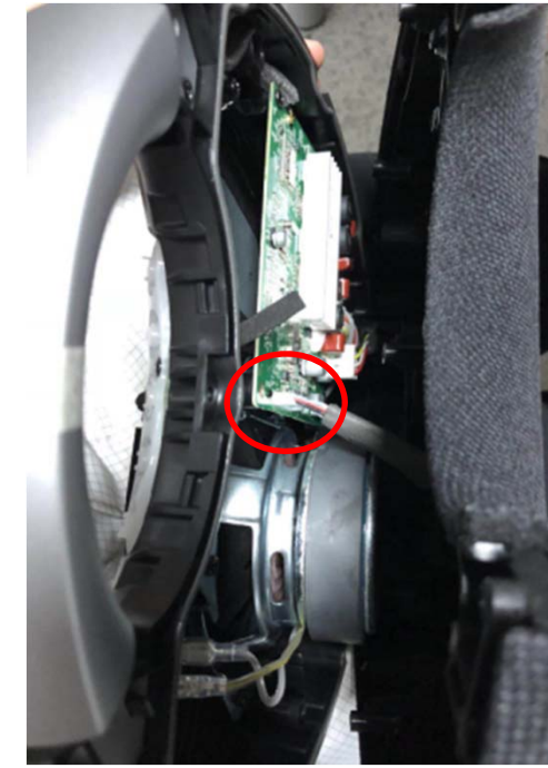
7. Unplug 1pcs cable on the main board, then take out cover
