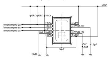
2. In case of setting I<sup>2</sup>C slave address of the sensor 1101001 \* Connect terminal ⑤ (AD\_SELECT) to VDD.
