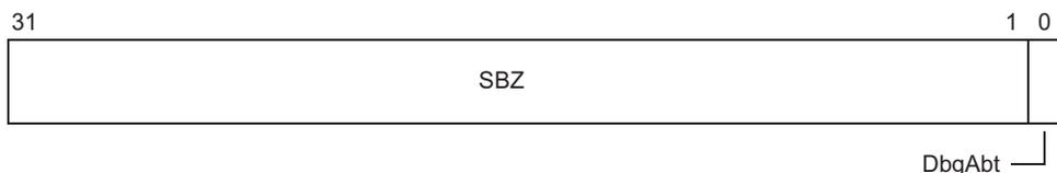
**Figure 8-9 Debug Comms Channel Monitor Debug-Mode Status Register**
