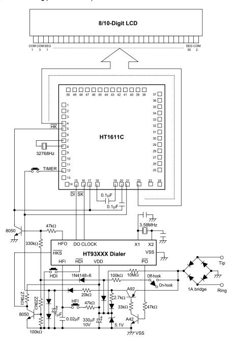
\* The IC substrate should be connected to VDD in the PCB layout artwork.
