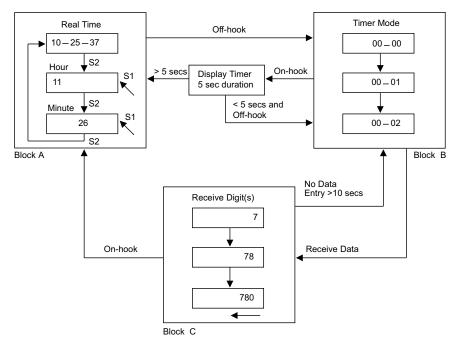
Note: Block A shows the switches S1 and S2 that are used for setting and selecting.
